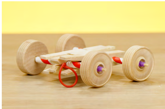
Prototype two mechanism: a rubber band is used to slingshot the car forwards.
