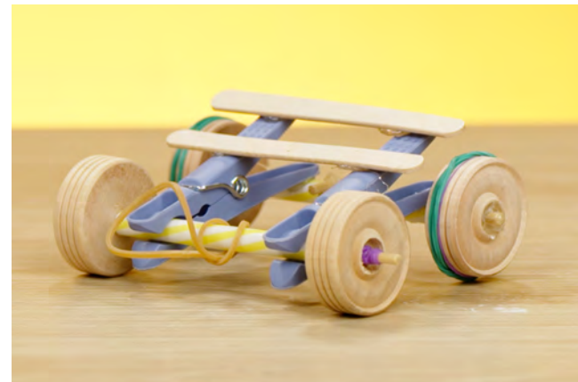
Prototype three mechanism: a rubber band is wound around the back axle and unwinds to make the car move.
